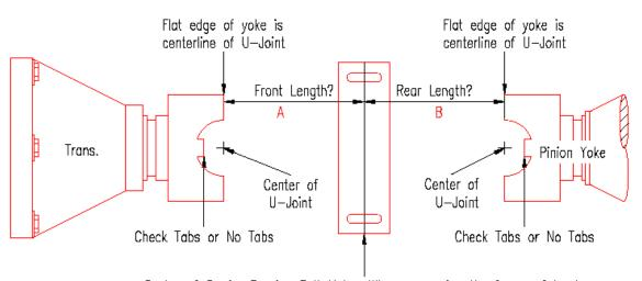
Centre of Carrier Bearing Bolt Holes. When measuring the frame of truck, most carrier bolt holes are slotted for some flex. <u>Go to middle of slots.</u>
